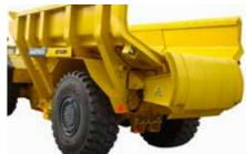
Minetruck MT431B can be equipped with a Teletram dump box, which pushes material off horizontally so it can be released in lowered areas with a low back height.
