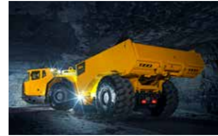
The smart, hydraulically operated tailgate works as a spill guard and supports the filling process with one extra side in the box.
