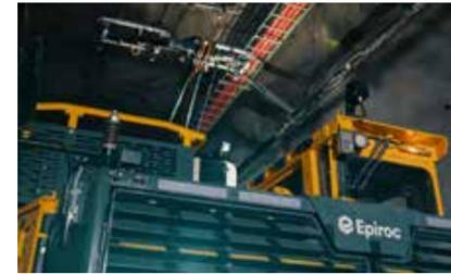
The pantograph on the Minetruck MT42 SG Trolley allows for continuous energy supply and dynamic charging.
