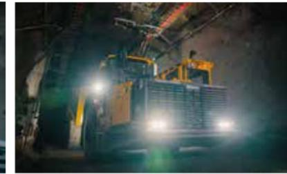
Thanks to an optimized battery capacity of 280 kWh, the truck can travel solely on battery power for up to 5 kilometers (3.1 miles) on inclines
