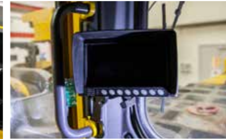
Dedicated camera displays in the direction of operation improves visibility, focus and by that safety.
