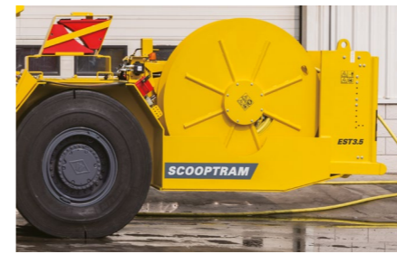
New strengthened cable with automatic tensioning cable reel is more wearable and extend service life.
