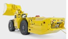
The patented cable reel control system automatically regulates tension to minimize wear on the cable and extend its longevity.
