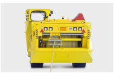
The horizontal cable reel enables a lower tension on the cable which will further improve the cables lifetime.
