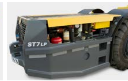
The loader's short, yet powerful frame and its lengthy wheel base makes the Scooptram ST7LP easy to maneuver and minimizes the risk of its back end hitting the ceiling.
