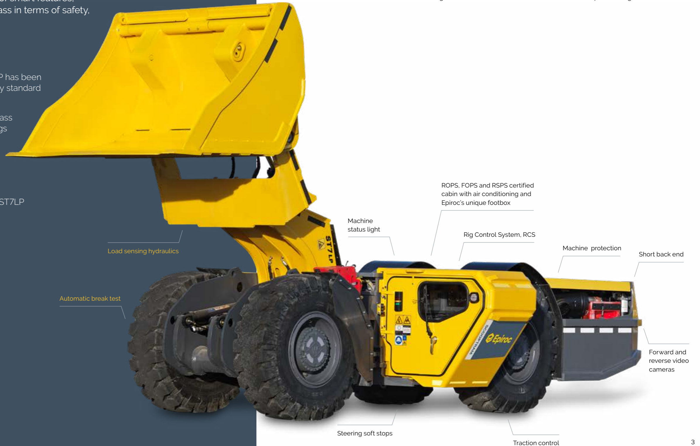
The loader's short, yet powerful frame and its lengthy wheel base makes the Scooptram ST7LP easy to maneuver and minimizes the risk of its back end hitting the ceiling.
