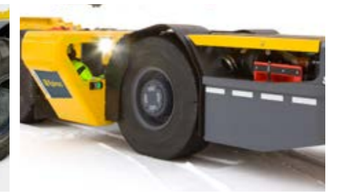
The Scooptram ST7LP includes traction control – a unique Epiroc feature that reduces wheel spin and tire wear in the muck pile to improve penetration and to enable one-pass loading.
