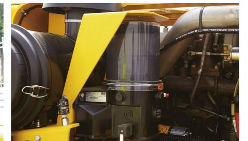
Automatic lubrication increases the MTBM (mean time between maintenance).
