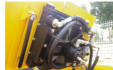
Individual hydraulic cooler serves for long service intervals and longer life of hydraulic components.
