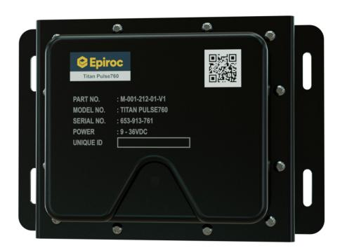
The Pulse760 is an ultra-wideband time-of-flight sensor used for precise ranging between vehicles and Epiroc's pedestrian tags, with an accuracy and range exceeding 80 meters. A high-accuracy GNSS receiver allows for accurate positioning in surface applications. The Pulse760 also features sub-GHz RF capability (868MHz or 915MHz) and is typically installed on the sides of a vehicle, with adaptations based on vehicle size.
