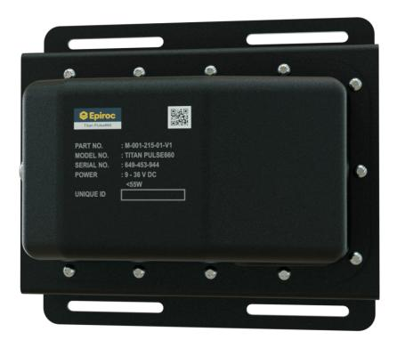
The Pulse660 generates a low-frequency (LF) magnetic field with object-penetrating capabilities. This magnetic field is created along a flexible cable transmitter, which allows for the generation of longitudinal fields that follows the shape of the vehicle. This is particularly useful for vehicles that can articulate as the magnetic fields will adjust with the articulation.
