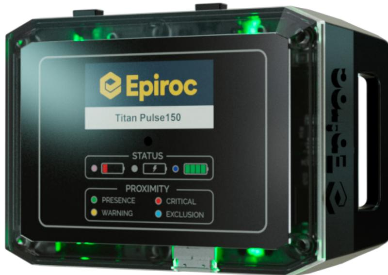
The Pulse150 features GNSS, LF magnetic field, and ToF capabilities, operating on the 868/915 MHz RF communication channel. It has an internal battery charged via USB-C, and includes LEDs and an audible warning to alert wearers of nearby vehicles.
