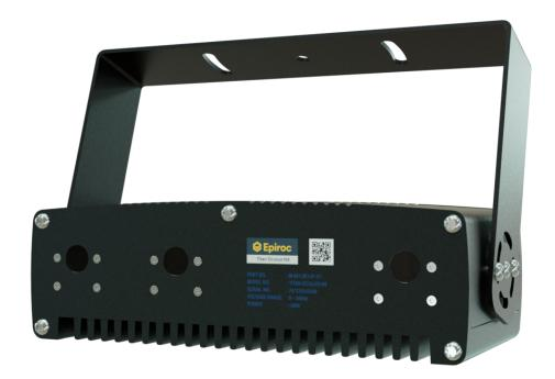
The Titan Oculus100 is a 1st generation Al Camera system designed for mining applications. It integrates a state-of-the-art Vision Processing Unit (VPU) to provide real-time object detection and ranging using stereo vision. This system extends the CAS capabilities, enabling the detection and ranging of both tagged and nontagged pedestrians and vehicles.
