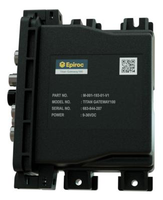
The Gateway100 serves as the interface for vehicle connectivity, executing collision avoidance algorithms, and managing system sensors. It includes an internal low-frequency transmitter for generating an exclusion field within the vehicle cab. With Wi-Fi capability and enhanced internal storage, it offers upgraded log-keeping capacity compared to previous systems.
