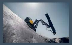
The SmartROC T30 R packs a powerful punch for a rig in this class. A COP SC19 HF rock drill with 160 or 250 cc and a compressor delivering 80 l/sec combined with the Volvo Penta diesel engine (105 kW/143 hp) ensures that together, you can handle the toughest
