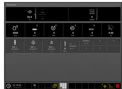
Performance: shows statistics about the machine and drilling consumables.
