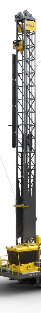
Robust "live tower" design can be raised and lowered with a full carousel and the rotary head at the top of the tower. State-of-the-art tower construction is designed to last for the entire life of the machine.
