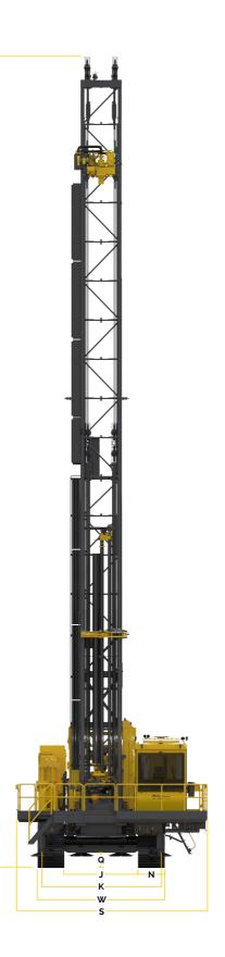
Approximate shipping dimensions for crated PV-271 E with 55 ft tower (actual dimensions will vary based on rig configuration).
