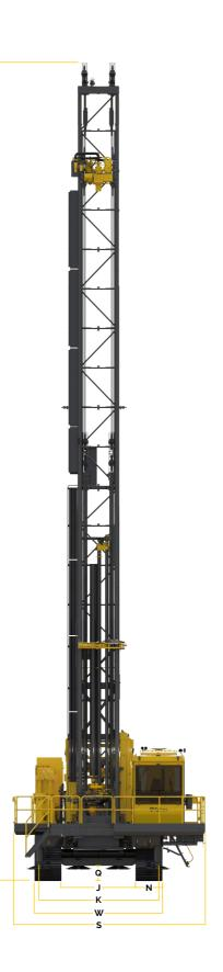
Approximate shipping dimensions for crated PV-271 XC E with 55 ft tower (actual dimensions will vary based on rig configuration).
