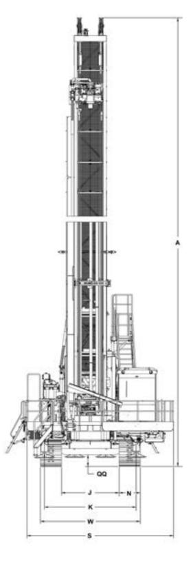
'Approximate shipping dimensions for crated PV-271 with 55 ft tower (actual dimensions will vary based on rig configuration).
